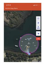
To demonstrate the process the anchor watch was set whilst Stoked was on her mooring (please disregard surrounding vessels). The first photo shows the set up with the anchor set due north at a distance of 20m and a comfortable 60m diameter safety zone. The second shows the established safety zone whilst the third photo shows the alarm activated as I rowed to shore — with the phone in the tender!
